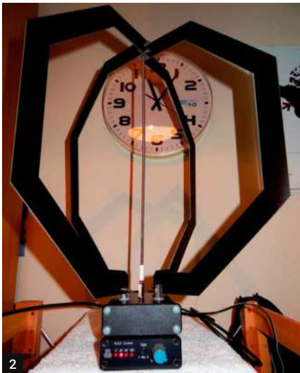
Fig. 1: The Reuter RLA3 in its pre-assembly state. Fig. 2: The RLA3A aerial, RLA 3 control unit, and fixed loop. Fig. 3: Close-up of the loop and control units (see also: Fig. 6). Fig. 4: The specially-coated loop blades. Fig. 5: Our review of the successor model, the Reuter RLA4, in RadioUser , May 2020: 18-20.
